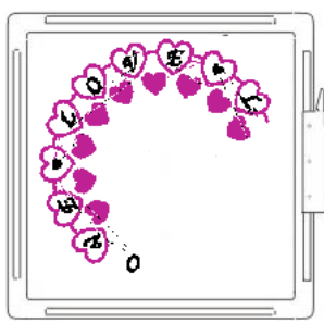
The hoop bracket is moved and the hoop frame rotated as needed to sew the various design segments.
